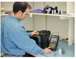
**Application:** Measurement of individual layers and total thickness in multilayer plastic automobile fuel tanks.
